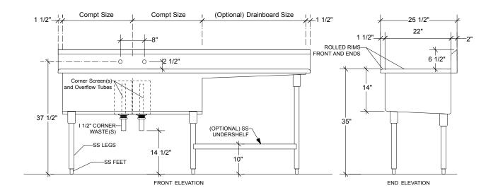
**Special Sizes:** Special size and gauge sinks and drainboards made to your requirements, submit rough sketch with sizes and specify gauges and optional extras required. A prompt quotation will be supplied and when order is placed, a shop drawing will be provided for your approval. QUEST sinks are an outstanding value.
