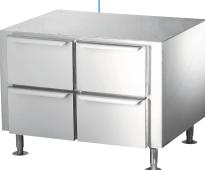
**Refrigerated Storage Base** 2 drawer 24" (305mm), 4 drawer 36" (914mm) or 6 drawer 48" (1220mm). Drawer concept adds operator efficiency. Drawers have heavy-duty self-closing slides and accept standard hotel pan inserts. All SS construction with "Cold Wall" refrigeration which helps prevent product from drying out. Remote compressor required.
